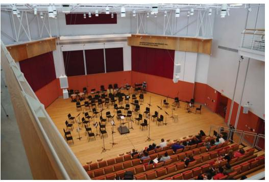
retracted. For symphony orchestra rehearsal and performance, ceiling height is the most important factor to ensure excellent acoustics. The 48' ceiling height is achieved by extending the main volume 12' above the existing roof, and by expanding the basement to the full building footprint. The orchestra stage is one storey below street level. Natural light floods the space from the clerestory created by the raised ceiling, which has a folded shape to distribute reflections evenly in the room.
